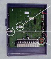
Integrated "Motor Rotation" switch to easily change motor rotation for though the wall mount, and other special applications
