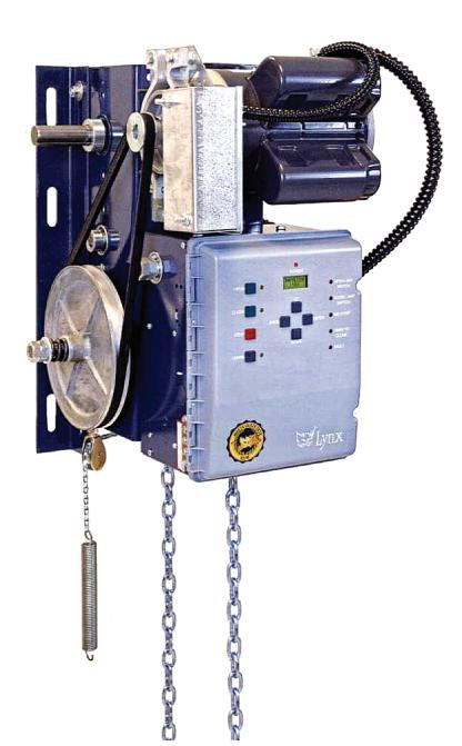
**MCJH** Standard/Industrial Duty jackshaft operator for high lift and vertical lift sectional doors, rolling doors and grilles. Durable Continuous duty highstarting torque motor with instant reverse and overload protection. Available in 1/2, 3/4, and 1 HP; single-or three-phase. MCJH is rated for up to 25 cycles per hour/80-90 cycles per day. It features our fully programmable LX 100 logic board, and heavy duty ball bearings on all line shafts.
