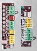
Includes 3 Monitored Safety Inputs to cover all entrapment points. (Add 3 more inputs with optional Expansion Board).
