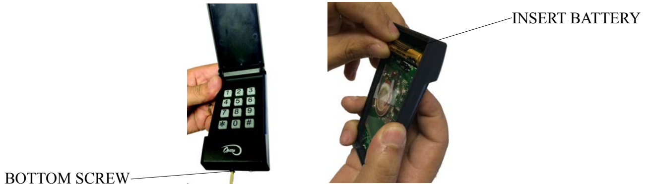
Figure 3 - KEYLESS042 Battery Installation
