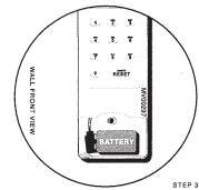
3 Replace 9V battery, then re-install battery cover.
