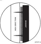
6 Insert bottom screw and tighten and re-install battery door.
