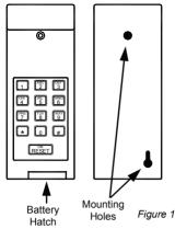
bottom screw. Install the screw leaving the head of the screw approximately 1/8 inch out from the wall. Slide the keypad over the screw and mark the position of the top hole. Remove the keypad and drill the top hole. Slip the keypad back over the exposed screw and finish mounting by installing the top screw. Refer to Figure 1.
