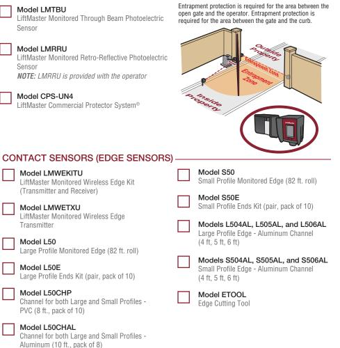
If utilizing a contact sensor as entrapment protection, one or more contact sensors shall be located on the inside and outside leading edge of a swing gate.
