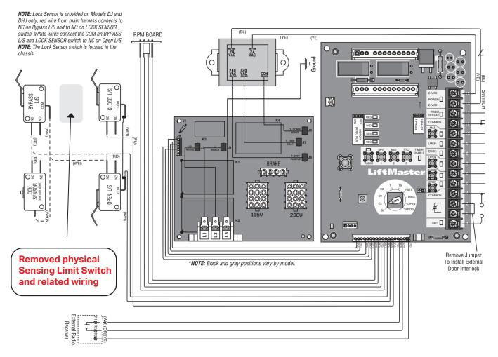
**NOTE:** 32 Vdc power supplied from White and Yellow wires located within the electrical box.
