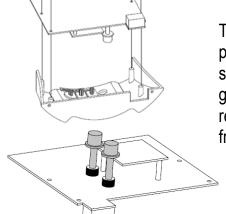
The only added steps from the board with the plastic to the new part number is to remove 4 screws attaching the plastic to the board, gently pulling the antenna wire through and removing and reinserting force control shafts from the original board onto the new board.
