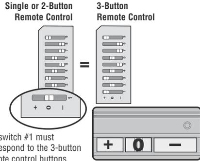
**Example:** If you are programming a single-button remote control to the middle button on the 3-button remote control, dip switch #1 in the single-button remote control MUST be set to "0" in order for both buttons to work.
