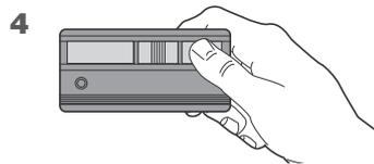
Repeat the steps 3-4 above with the yellow button on the remote control and the receiver Smart/Learn button “B” to program the CLOSE mode; and again with the green button on the remote control and the receiver Smart/Learn button “C” to program the OPEN mode.
