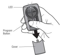
Press and release the button. When the LED stops flashing, continue to press and release the button until a click is heard from the garage door opener, a light on the garage door opener blinks, the garage door opens/closes, or a beep is heard from the gate operator (maximum 18 times).
