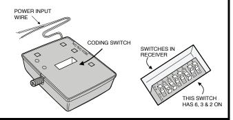
**STEP 3** Connect receiver to 24V power. Connect the white power input wires to the 24V and Common terminals on the gate operator. If using DC power, gold wire (+), silver wire (-).
