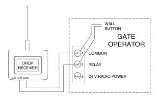
**STEP 5** Test receiver. Be sure gate area is clear. Activate each transmitter and verify that the receiver triggers the operator.
