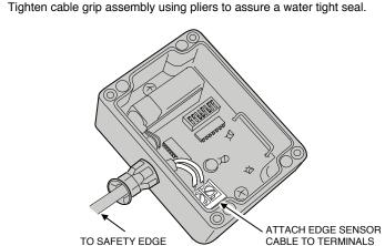
Attach Cable. Attach safety edge cable to terminals as shown.
