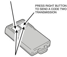
PRESS BOTH BUTTONS TO SEND A CODE THREE **TRANSMISSION**
