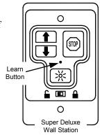
**Step 5:** The work-lamp on the MVP will turn off when a valid PIN has been learned.
