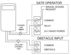
STEP 5 Connect receiver to power. Connect the red power input wire to the 24VDC radio power and the black wire to the common terminal on the gate operator. Alternately connect wires to a 12-24 VAC transformer.
