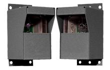
The IRB-325 thru beam photoeye is an external entrapment protection device type B1, non-contact sensor for use with automatic gates and doors. The photoeye provides a signal to the gate or door operator that the beam is or is not obstructed. The IRB-325 operates up to 65 feet and is UL325 compliant with operators that require normally closed (NC) monitoring.
