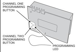
**STEP 5** Program receiver. Momentarily press the receiver's program button (channel one or two). The red programming LED will light if there's room in the receiver's memory for another transmitter (10 maximum per receiver). The LED stays on for about 5 seconds. A transmitter must be entered while the LED is on. Press the desired transmitter button. The LED will flicker indicating that the receiver has accepted the transmitter.
