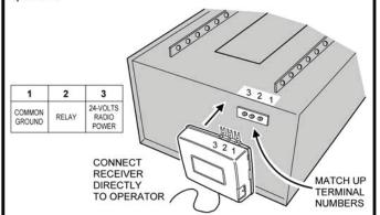
STEP 2 MDR2/MDRM2 Two-channel Receiver Installation. Connect the receiver to the operator as described in the previous step. The channel-two pigtail wires can be connected to the operator's light toggle terminals or to an external device.
