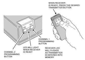
**STEP 6** Add additional transmitters. Repeat Step 5 for each transmitter used with this receiver. Be sure to press the receiver's program button *each time* a new transmitter or a different transmitter button on a multi-button transmitter is pressed.
