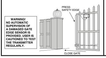
**STEP 8** *Test Safety Edge.* Test safety edge connection by pressing the safety edge. The power light should come on.
