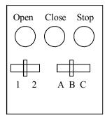
**Open, Close & Stop transmitter to control 6 Doors.** Match dipswitches 1, 2, 3, 4, 5 & 8 on both transmitter and receiver. Set the 6th and 7th dipswitch in the open/close/stop receivers accordingly.
